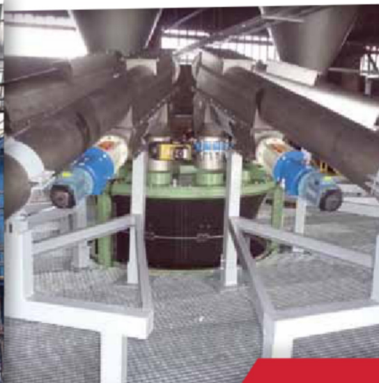
DOSING SYSTEM WITH HYPALON HOPPER FOR BATCH INTEGRITY
