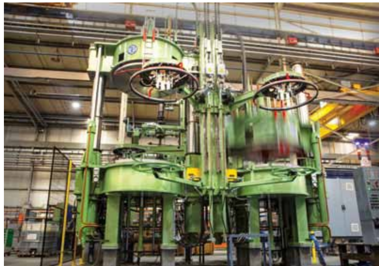
65" Floating Column Hydraulic Press
