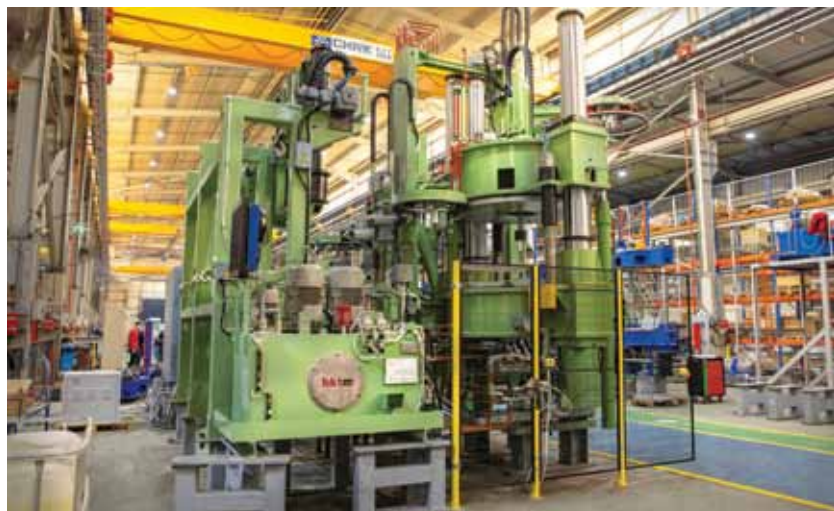
65" Floating Column Hydraulic Press
